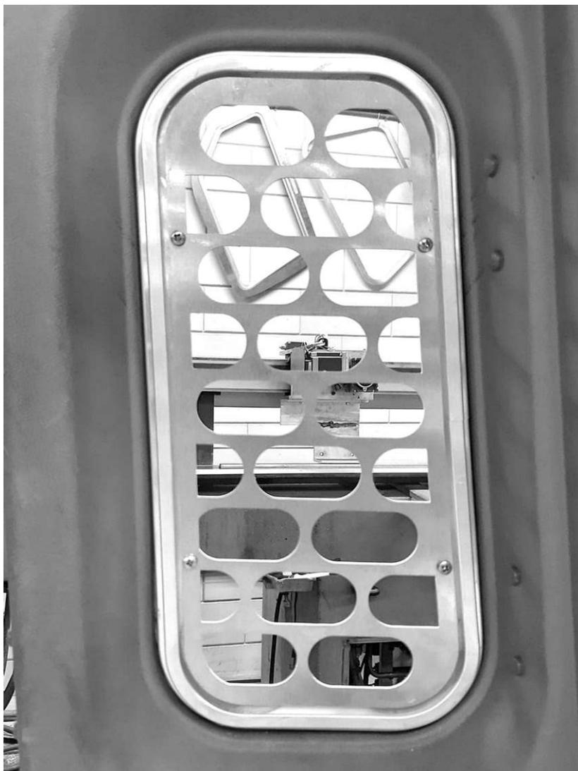
*Figuur 1 Quarter window with inner lining.*
